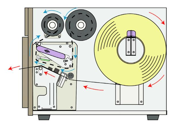
Figure 7-5c, Printer Loading Diagram
